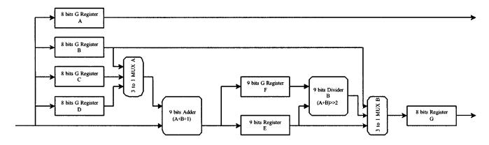
Fig. 9. Architecture of the interpolation pixel generator.
